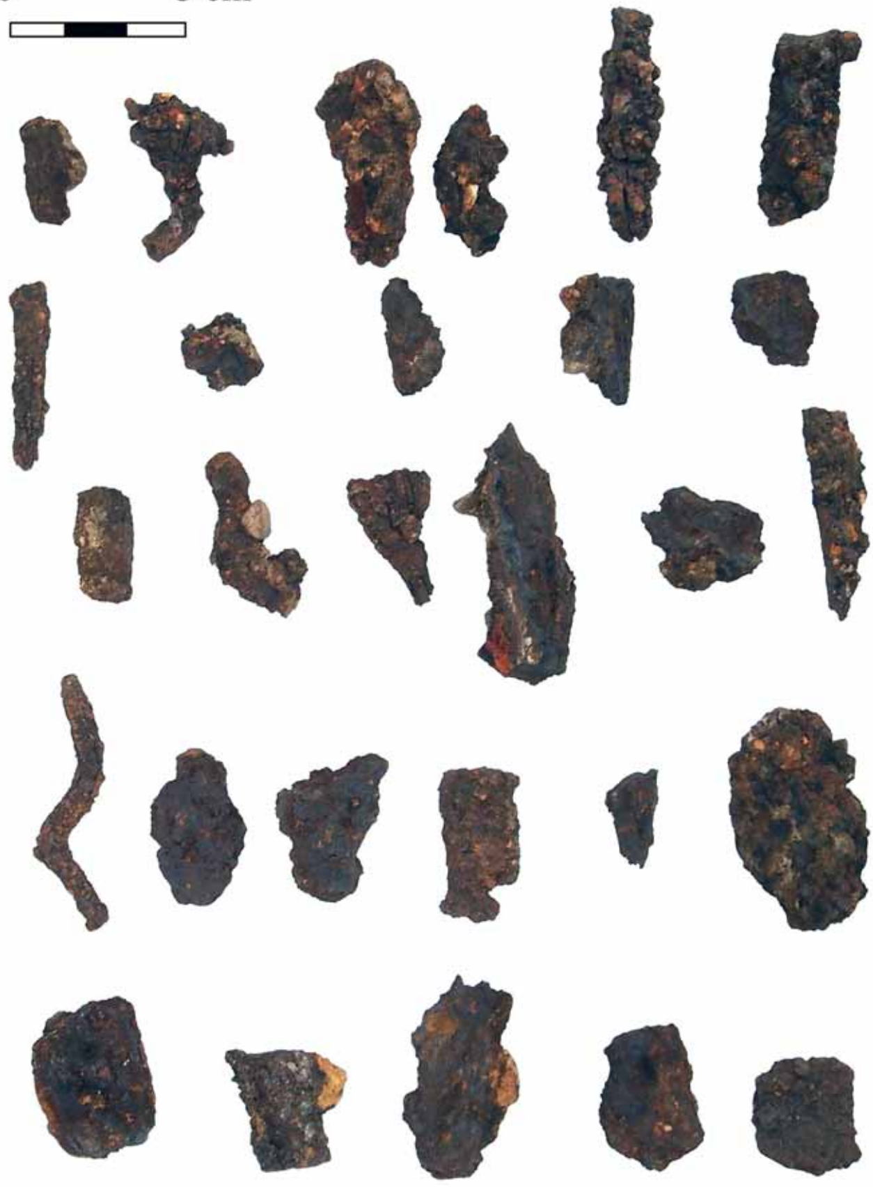
Figure 6. Samples of iron waste from 3 th -1 st century BC forges, from Cucini (2015, Fig. 22).
